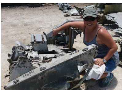
Image to the left: Member pointing to ID plate of cockpit section of the P38 lightning aircraft. (S/N: 1911940, LOCKHEED AIRCRAFT CORP, BURBANK CALIFORNIA)
